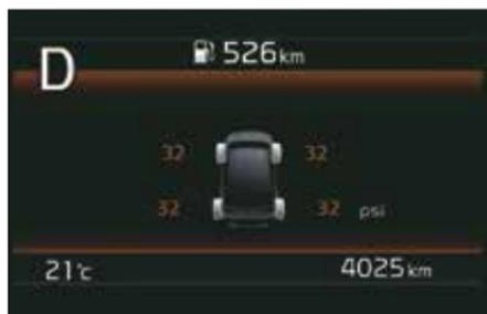
Continuously monitors air pressure in each tyre and alerts you in case of a drop below recommended levels while driving
